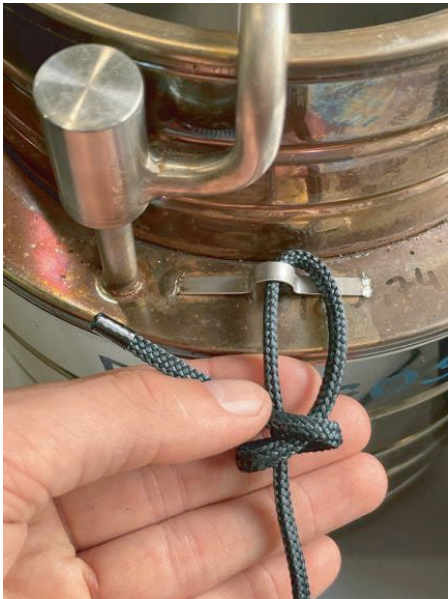
With the working end of the cord, make a turn at the beginning of the loop.
